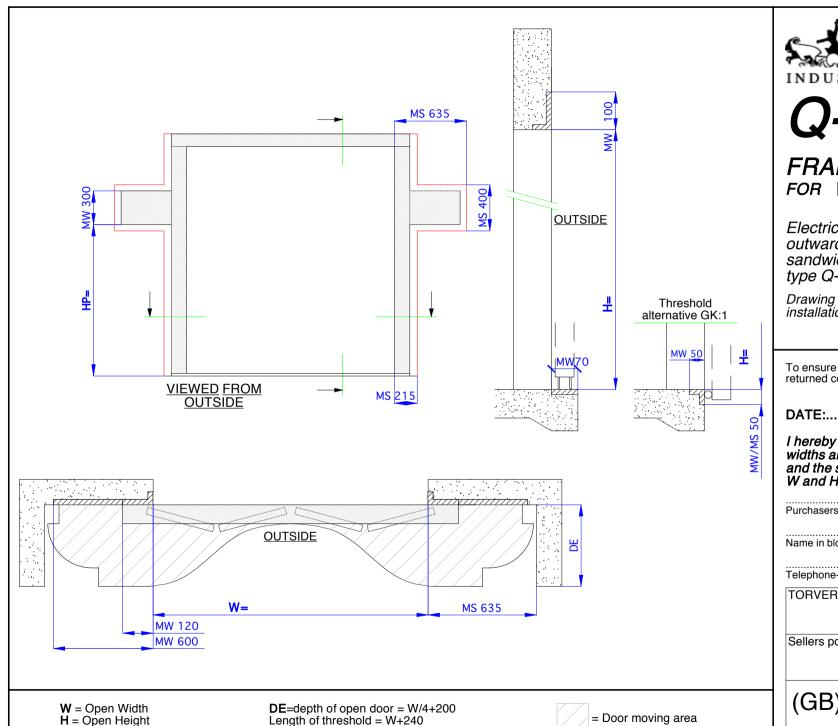
**MW** = Minimum steel Width **MS** = Minimum Space
